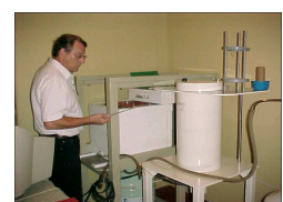
A sample is placed into the \gamma -detector for the \gamma -analysis
