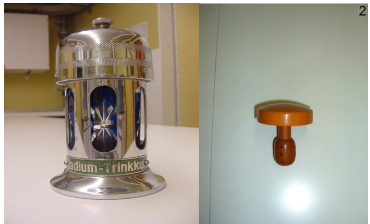
Device of a Radium-drinking-cure (left) and the radium-source placed in the cap of the device (right).
